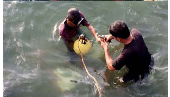
Deploying a current meter to measure tidal current speed and direction in Puerto Azul, Ternate, Cavite
