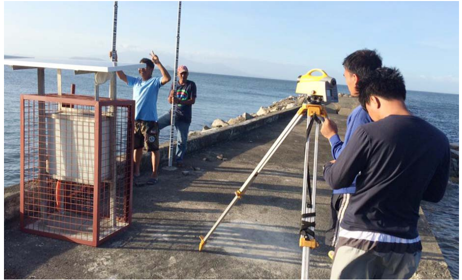
Conducting tidal leveling in Puerto Azul, Ternate, Cavite
