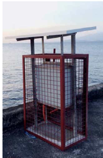
The CDS pressure-type tide gauge installed in Puerto Azul, Ternate, Cavite
